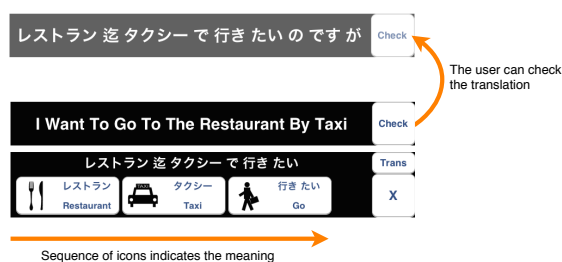
Fig. 3. The process of communication by using the picoTrans system. The sentence is a little more complex than that in Figure 2 to illustrate the additional expressive power of our approach. The picoTrans system displays the icon sequence, together with a translation of the user’s intended meaning. This translation can be checked in the target language by referring to the icon sequence, and in the source language by referring to a back-translation.
